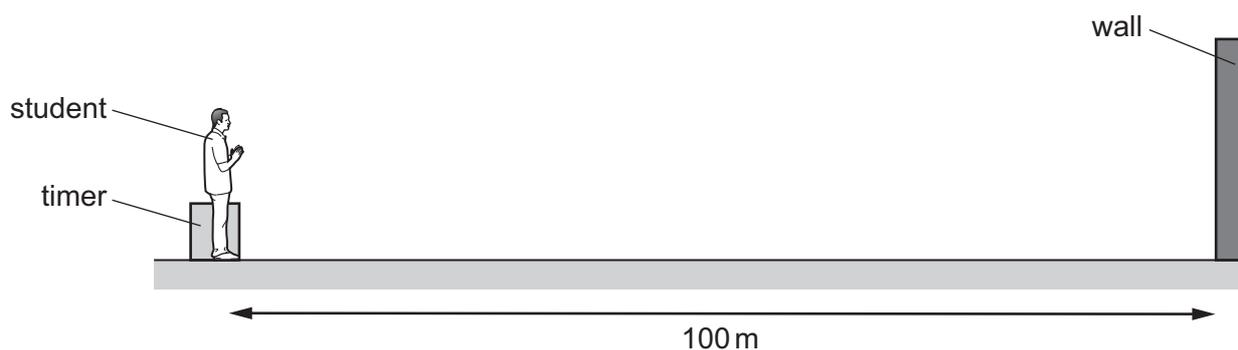
An electronic timer detects the echo of the sound 0.60 s after it is made.
